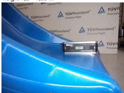
Fotografia / Photo 5 2_324_xxx HDPE wave slide for assembly height 1,2 – 1,25 m
