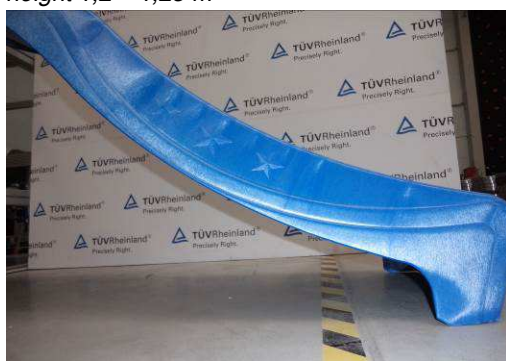
Fotografia / Photo 7 2_324_xxx HDPE wave slide for assembly height 1,2 – 1,25 m
